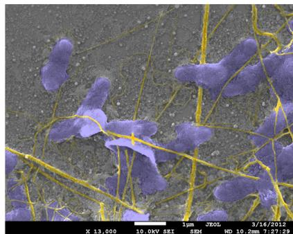
False color SEM image depicting cells (purple) and fibers (yellow). Fiber width ranges from 20 to 200 nm.
