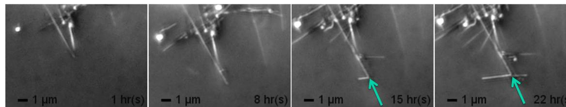
A series of images showing growth of arsenic sulfide nanofibers as observed with bright field microscopy at 45°C. Elongation after the bend in the fiber indicates growth is from the fiber's tip. Fiber morphology remains consistent at different growth temperatures.
