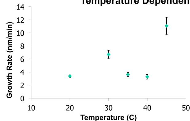
Average growth rates over the first 24 hours at various elevated temperatures. Preliminary data show an increased growth rate at higher temperatures, and further experiments will be conducted to verify. Error bars shown represent two standard errors.
