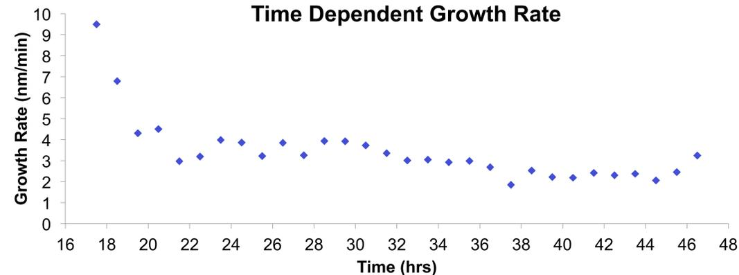
Binned averages of 20°C growth rate of more than 50 arsenic sulfide nanofibers. Decay over time suggests dependence on arsenic and sulfur concentration. Growth rate remains roughly constant at later times, implying that arsenic and sulfur concentrations have become limiting.
