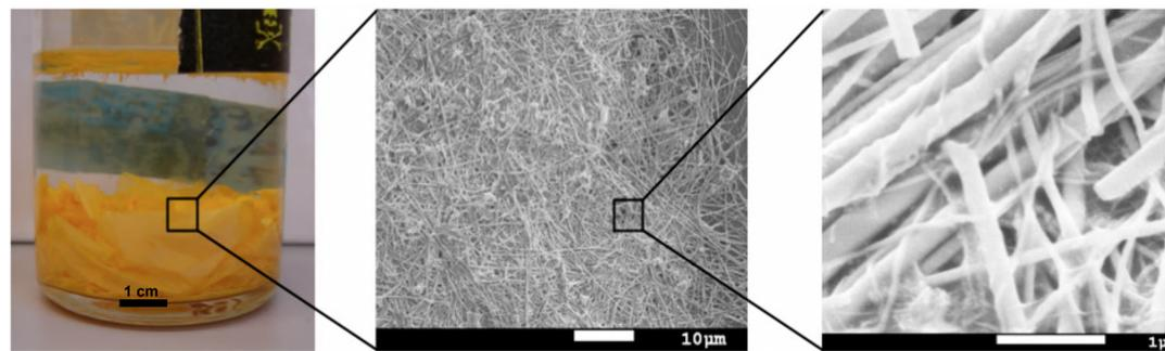
(A) Photograph of bright yellow macroscopic sheets of  $\text{As}_x\text{S}_y$  that precipitated from solution. (B) SEM image of the sheets composed of nanofibers. (C) A higher magnification SEM image showing individual nanofibers.
