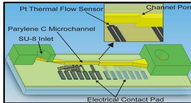
Schematic of the microfluidic platform for focal stimulation
