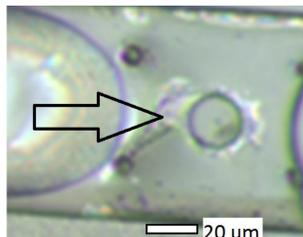
A pore in a microchannel (3 different pore sizes – 5, 10 and 20  $\mu$ m).
