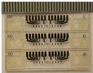
A microfluidic chip (1.5x1 cm) designed with 3 microfluidic channels (4x100 $\mu$ m) each with a pore in the middle of the channel.
