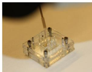
A microfluidic platform is packaged with a custom made acrylic jig and glass capillary tubes are inserted through the PDMS gaskets, carefully aligned to match inlet and outlet ports of the device.
