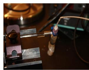
A 3-way valve connecting a glass syringe, a plastic syringe and PEEK tubing is connected to a precision glass syringe driven by a syringe pump.
