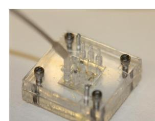
The other end of the PEEK tubing is connected to the assembled microfluidic platform.
