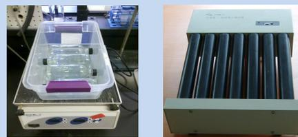
Figure 3. Initial shaker device and roller mixer
