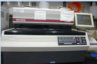
Figure 1. Beckman 6000 Liquid Scintillation Counter
