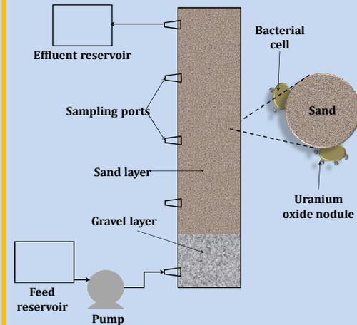
Figure 5. Schematic of bioremediation testing column
