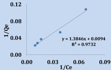
Figure 4. Langmuir adsorption isotherm for uranium using shaker
