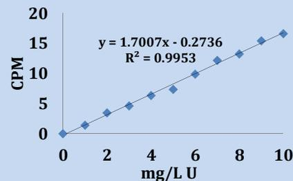
Figure 2. Calibration curve from 1 mg/L U
